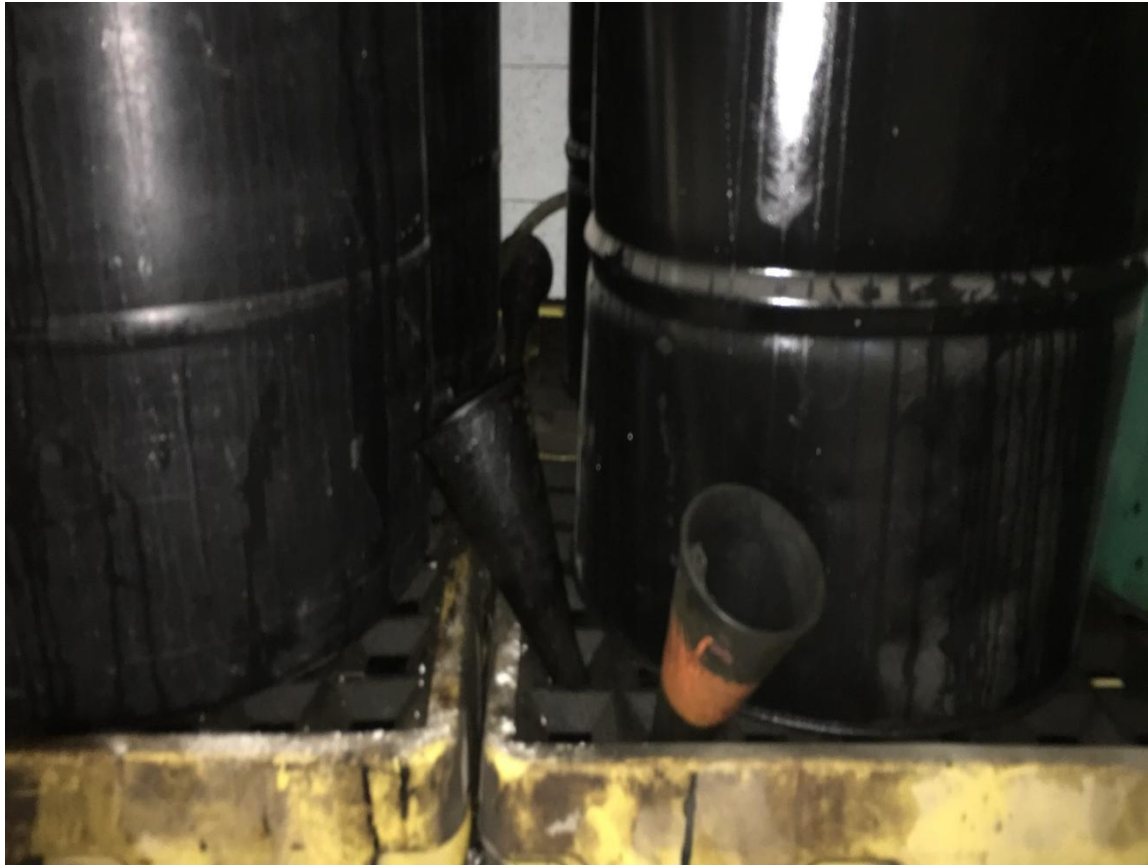
IMPROPER USE OF SPILL CONTAINMENT PALLET
