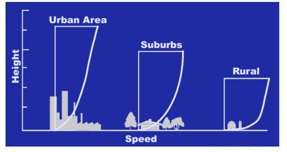
Tip: Check the vectors used to define surface roughness length for worst-case wind directions
