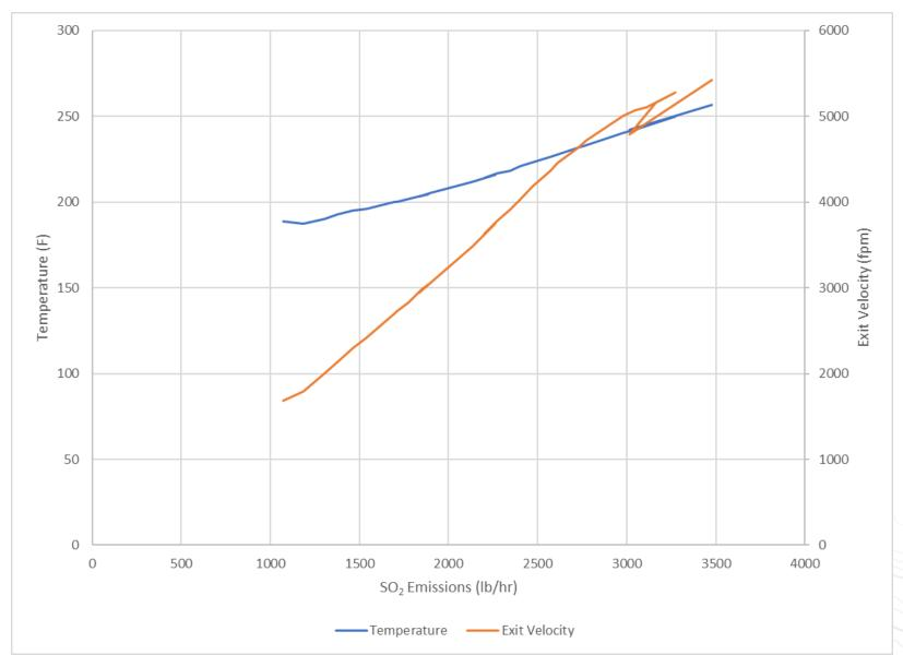
Utilize stack flow/temperature data that corresponds to the emissions modeled
